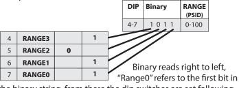
the binary string, from there the dip switches are set following the description ordering using the binary string for the desired setting. 13. Inspect LCD for readings. LCD toggles between sensor A reading, sensor B reading, and PSID reading.
